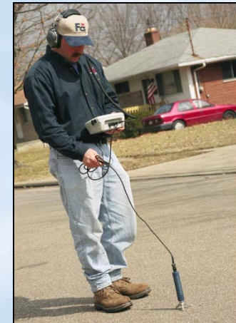
Traditional leak detection survey
